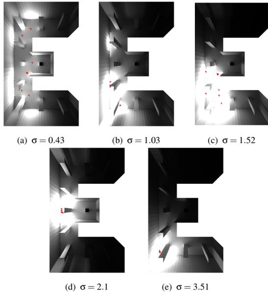
Figure 2: Different radiosity distributions in the “E” scene ( $n=24736$ ), and their  $\sigma$  values. Red patches are the emitters.
