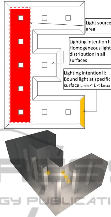
Figure 1: A top-view scene with a lighting intention configuration example (top) and a possible solution for positioning four light sources (bottom).
