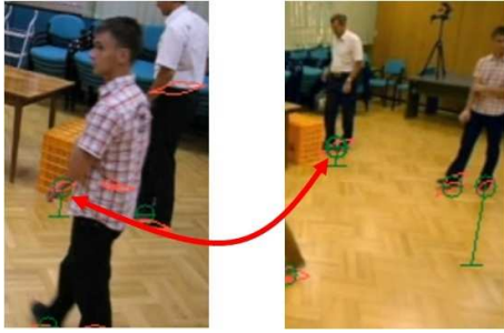
Figure 3: Candidate pixels can appear on arms or on foreground artifacts, and also cones corresponding to different feet can intersect.
