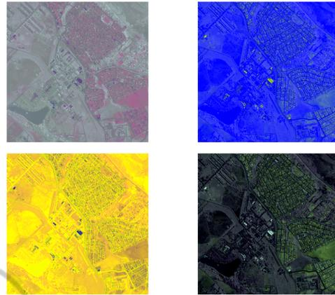
Figure 1:  $p=[1/2, 1/2, -1/2, -1/2]$ ,  $q=[-1/2, -1/2, 1/2, 1/2]$ ,  $\gamma = 0.6$ ; bands 1 (in R), 3 (in G), 4 (in B).  $p=[1/2, 1/2, 1/2, -1/2]$ ,  $q=[1/2, -1/2, 1/2, 1/2]$ ,  $\gamma = 1.0$ ; bands 1, 2 and 3.  $p=[1/2, 1/2, 1/2, -1/2]$ ,  $q=[-1/2, 1/2, 1/2, 1/2]$ ,  $\gamma = 1.0$ ; bands 2, 3 and 4.  $p=[1/2, 1/2, 1/2, -1/2]$ ,  $q=[1/2, -1/2, 1/2, 1/2]$ ,  $\gamma = 1.0$ ; bands 1, 2 and 4.
