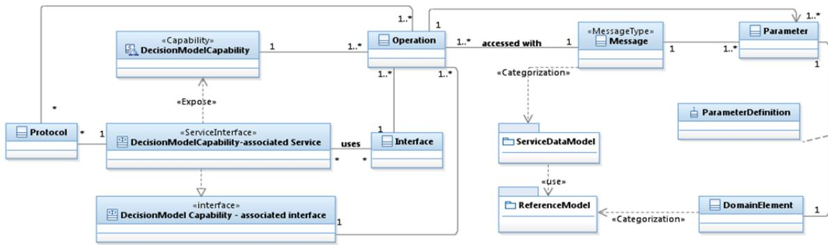
Figure 7: Service Specification Meta-model.
