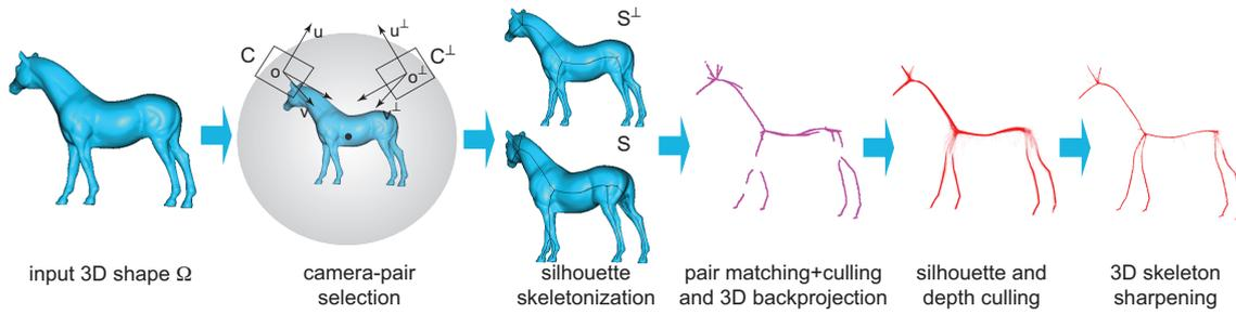
Figure 1: Curve-skeleton probability computational pipeline.
