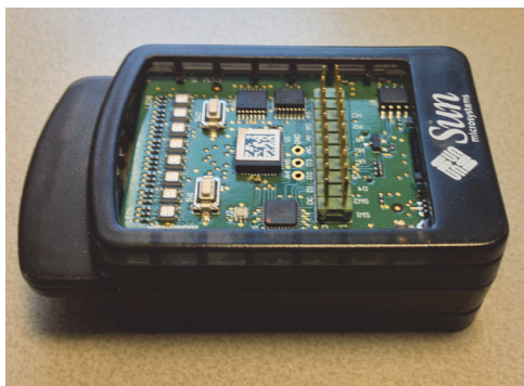
Figure 2: The SunSPOT, developed by Sun Microsystems, and which is used as prototyping platform for this project.
