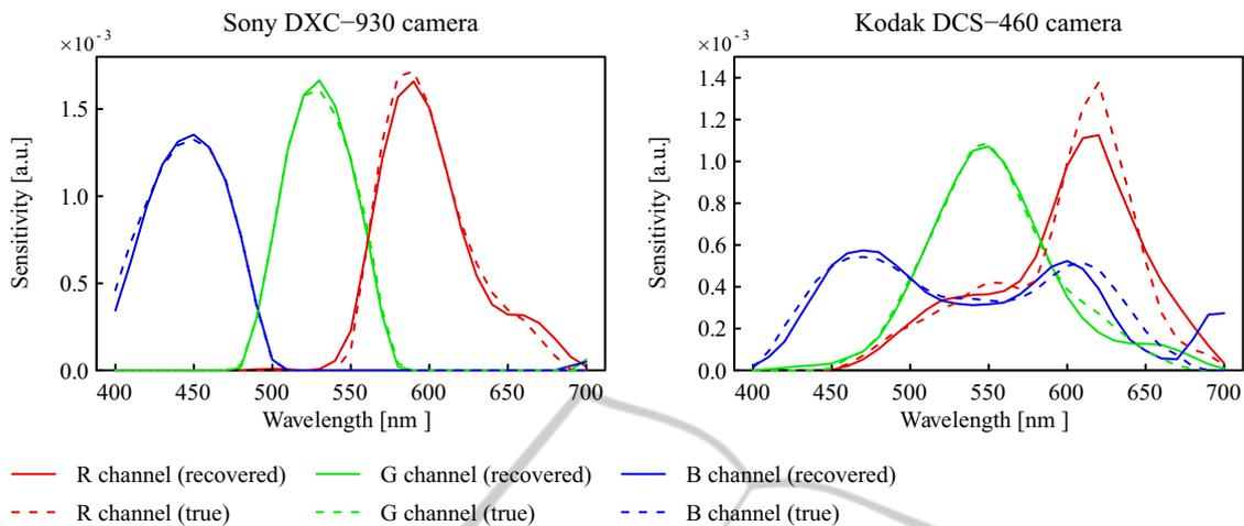
Figure 4: Results of the spectral sensitivities by the proposed method. Nonlinear camera model (the gamma characteristic 2.2) are used and 1% noise ( $\sigma = 0.01$ ) was added to the synthetic sensor response data.
