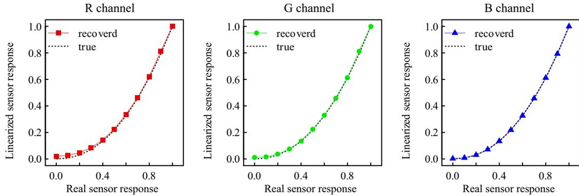
Figure 3: Results of the estimated linearization functions. The settings correspond to those in Table 2.
