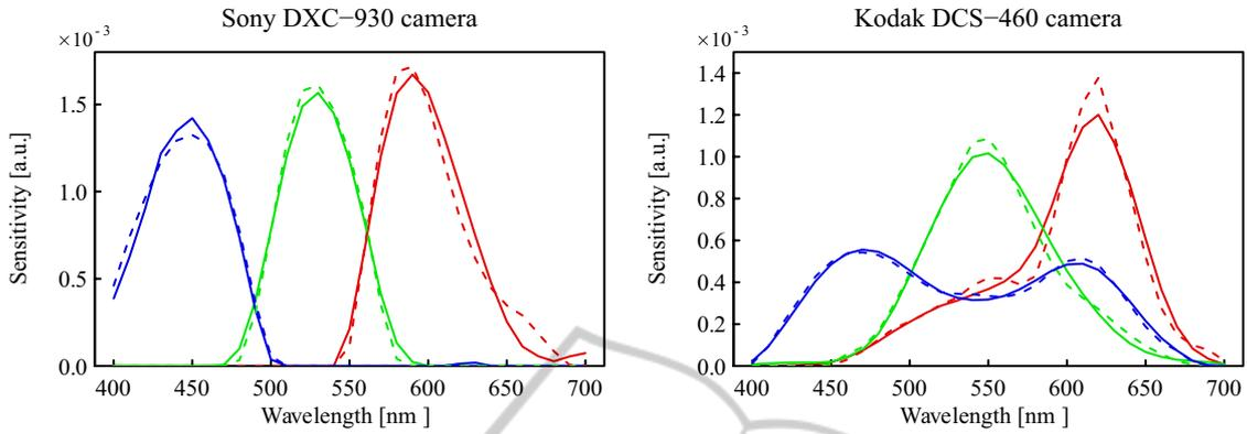
(ii) Method A: Minimizing the sum of the squared absolute errors of sensor responses with the constraints of nonnegativity and modality and Fourier basis
