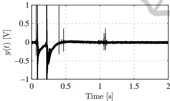
Figure 6: First 2 [s] of recorded accelerometer signal shown in time domain. The signal is perturbed with noise over the whole measurement. The noise is assumed as i.i.d Gaussian noise,  $\sigma = 1.6e-4$ . The searched resonators both appear in the time domain at approximately 1.1 [s] after start of the filling phase. The exact time point is estimated with the correlation coefficient computation.
