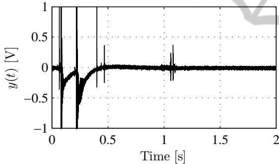
Figure 6: First 2 [s] of recorded accelerometer signal shown in time domain. The signal is perturbed with noise over the whole measurement. The noise is assumed as i.i.d Gaussian noise,  $\sigma = 1.6e-4$ . The searched resonators both appear in the time domain at approximately 1.1 [s] after start of the filling phase. The exact time point is estimated with the correlation coefficient computation.
