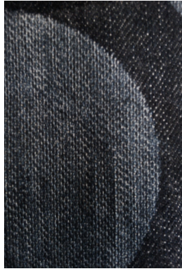
Figure 3: Line effect on 30 dpi laser engraving.
