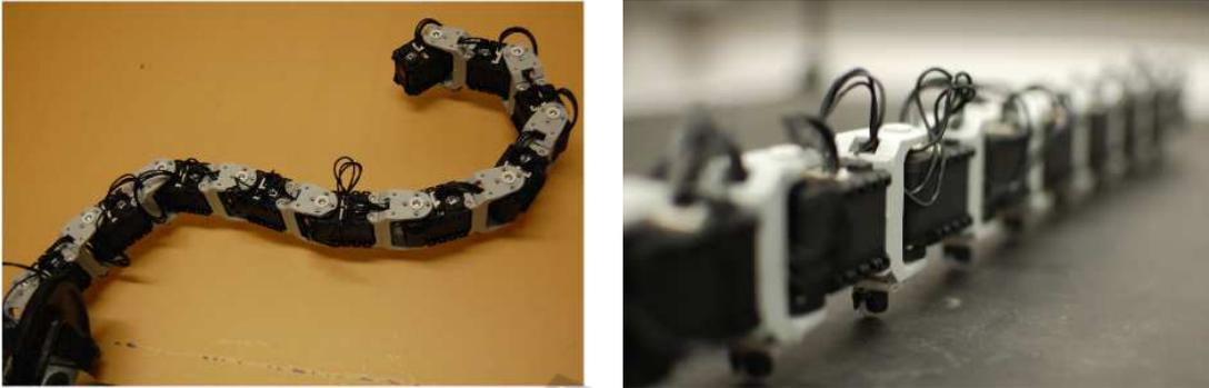
Figure 1: A planar tentacle robot with ten links.
