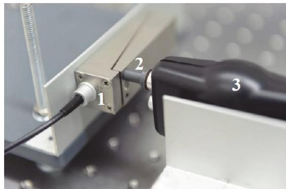
Figure 3: Representation of the mechanical structure of the test setup I. 1-ACT. 2- PVC interface. 3- AP.
