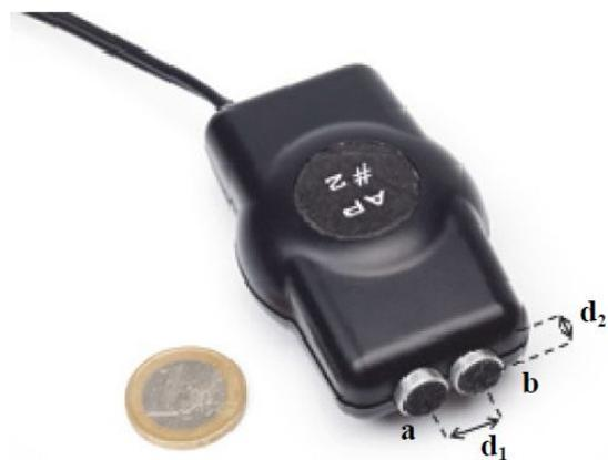
Figure 1: Representation of the double headed probe. a- Microphone 1; b- Microphone 2; d1-distance between transducers centres: 11mm; d2- sensors height: 2mm.
