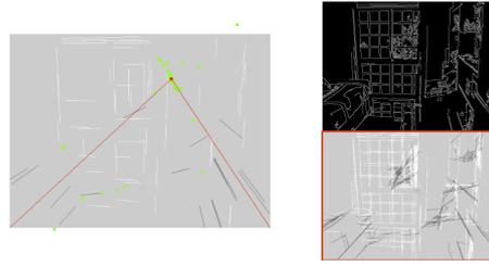
Figure 5: Vanishing Point analysis for Figure 4. On the top right: Canny filter analysis. Bottom right: detected line segments, oblique lines are in black. Left: main line intersection points in green and main vanishing point detected using clustering nearest neighbors.
