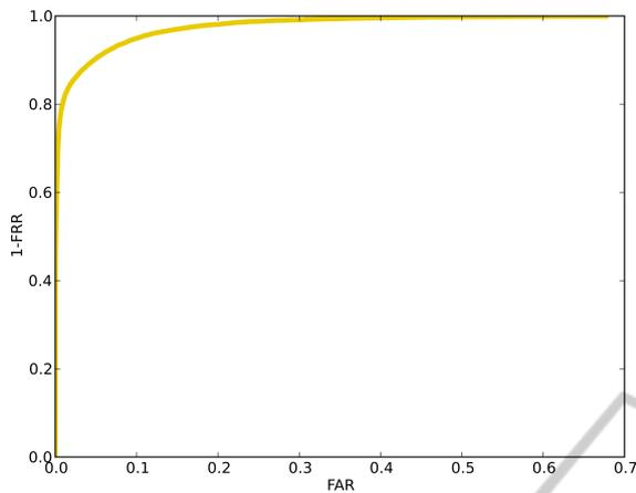
Figure 4: ROC curve for the  $m = 5$  best case scenario;  $m$  denotes the number of waves used to compute the mean wave.
