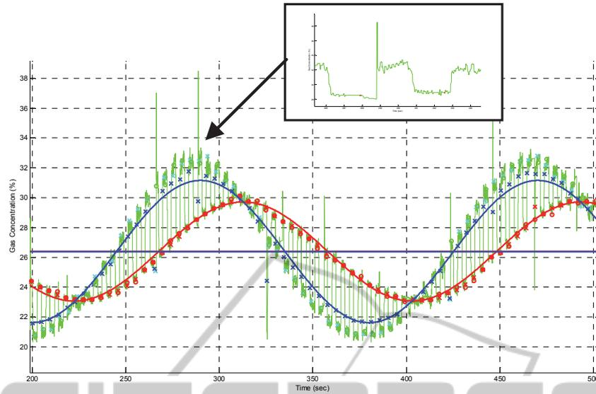
Figure 1: An example of  $O_2$  signal collected in an inspired sinewave lung function test. Green line is the measured  $O_2$  signal. Blue marker and line are the mixed inspired concentration and sinewave. Red marker and line are the end-expired concentration and sinewave. The more attenuated the end-expired concentration, the greater the dead space, lung volume, or pulmonary blood flow.
