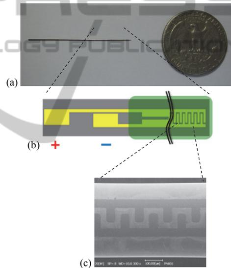
Figure 2: Configuration of the electrical acupuncture needle passivated by parylene C: (a) fabricated electrical acupuncture needle, (b) schematic of the Ti/Au bipolar electrodes (bright yellow), the conventional acupuncture needle (dark gray) and parylene C electrical insulation layer (translucent green), and (c) SEM image of a part of the IDE.
