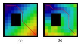
Figure 1: Paths on a 2D space from an initial cell at the bottom-right corner to the goal cell at the top-left one, computed with the NF1 function (a) and with the NF1 function modulated by the clearance (b).
