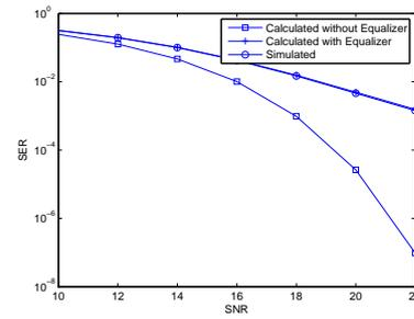
Figure 2: SER comparison with the following parameters:  $d = 1$ , the step-size parameter  $\mu = 0.00005$ , the averaged results were obtained in 100 Monte Carlo trials where 128000 symbols were produced for each trial.
