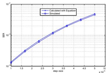
Figure 4: SER comparison with the following parameters:  $d = 1$ ,  $SNR = 20$  [dB], the averaged results were obtained in 100 Monte Carlo trials where 128000 symbols were produced for each trial.
