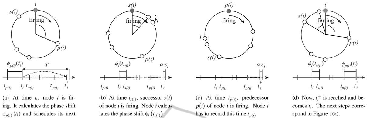
Figure 1: Snapshots of the desynchronization process from node  $i$ 's point of view. Nodes move clockwise on the circle at frequency  $f = 1/T$  with period  $T$ .
