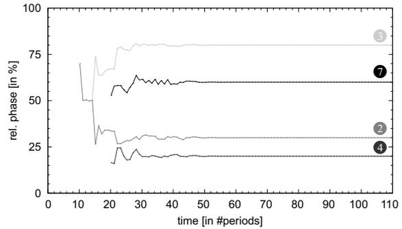
Figure 4: Simulation of  $M_7$  (about 110 periods since the start up of node 1 at period 1),  $\alpha = 0.95$ ,  $\rho = 0.25$ , point of view: node 1.
