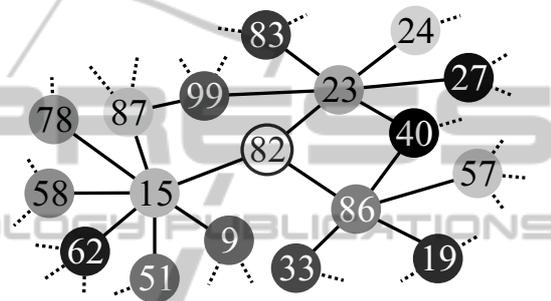
Figure 5: One-hop and two-hop neighborhood of node 82 of topology  $R_{100}$ , consisting of the set  $N = \{1, \dots, 100\}$  of nodes.
