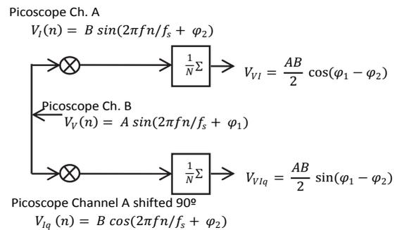
Figure 6: Schematic of Phase-sensitive Demodulator implemented in the EIS system.
