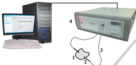
Figure 2: Schematics of the EIS OEM system – 1) Biologic sample; 2) electrodes; 3) short coaxial cables; 4) EIS system conditioning unit and acquisition system, with the PicoScope®3205A incorporated; 5) laptop/PC.
