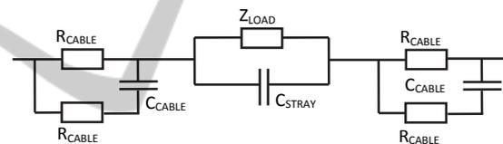
Figure 5: Equivalent electric circuit of all parasitic elements affecting impedance measurements of a load,  $Z_{LOAD}$ . The effect of the stray capacitances from cables,  $C_{CABLE}$ , is minimized by the driven shield. Other stray capacitance effect,  $C_{STRAY}$ , due primarily to the phase shift of amplifiers, can be minimized by software.
