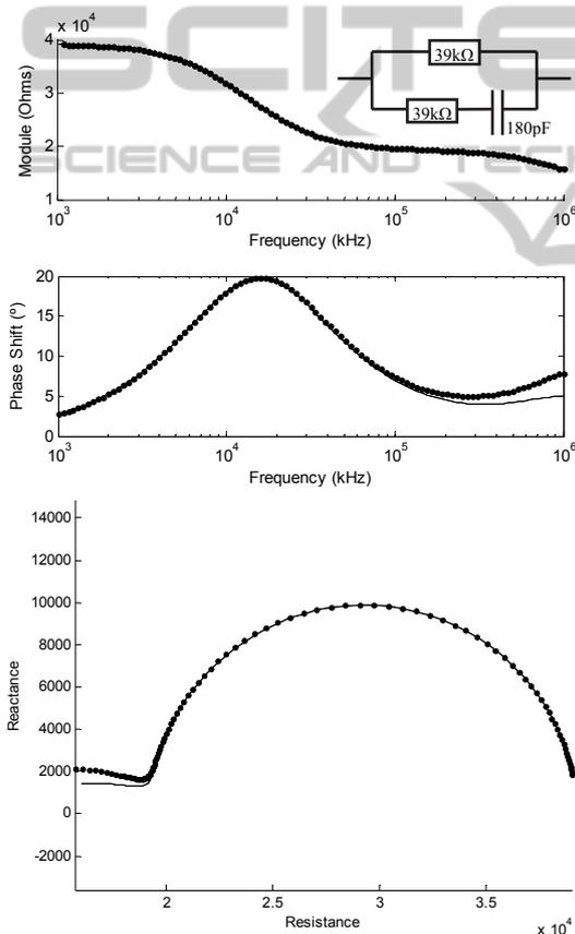
Figure 4: Bode and Cole-Cole diagram showing the reduction of cables capacitive effect by the application of the driven shield technique. The voltage mode excitation was used to analyze the circuit at the right top. The reduction is more noticeable at high frequencies where the capacitive effects have more influence.
