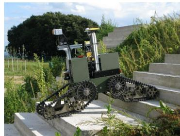
Figure 1: The Telemax robot is a tracked platform with four actuators. It is able to traverse rougher terrain and to overcome more obstacles than many fixed-chassis robots.
