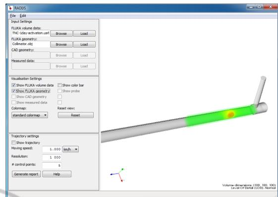
Figure 2: A screenshot of the software's Graphical User Interface, showing the volume rendering of a radiation dose simulation in the TNC tunnel at CERN. The geometry of the cavern is shown as well and is partly translucent to be able to have an overall view on the situation.
