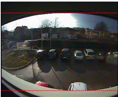
Figure 3: An example of severe lens distortion. Red dotted lines serve as a straight reference.
