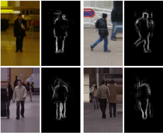
Figure 2: Product of the likelihood provided by SVM with the gradient of the image for 4 examples. These values used in equation 1 give accurate clues on the silhouette contour.
