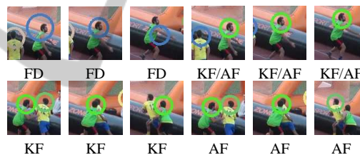
Figure 4: Examples of tracking using different predicted position techniques. Using a simple finite difference scheme (FD) lacks in presence of noise, while both kalman filter (KF) and adaptive filters (AF) can deal with it. When occlusion occurs, AFs performs better when recovering a moving object, while KFs obtain better results tracking the stopped one.
