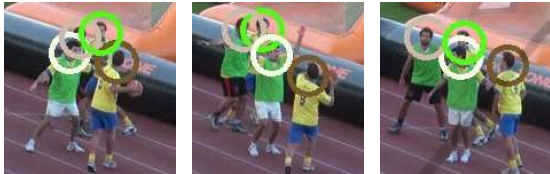
Figure 5: Partial occlusion example. The system is able to detect every person in the collision, even when sudden orientation changes occur.
