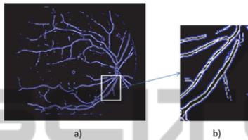
Figure 1: a) Modified Kirsch filter resultant image where the blue and white pixels represent negative and positive gradient values, respectively. b) One section image expanded version of a).
