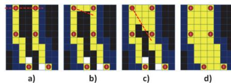
Figure 3: RA “filling” state graphical representation. It analyses the pixels located between each pair of two points belonging to its contour by determining the line linking these two points a) – c); d) all the points that are inside the contour, with grey level value similar to the contour average grey level value, are added to the region.
