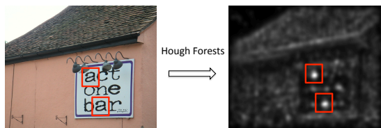
Figure 2: Generalized Hough transform for character “a” by using Hough forests (the image is taken from the ICDAR 2003 dataset).
