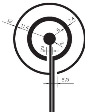
Figure 1: Dimensions (mm) of the concentric ring electrode to be implemented in the array.
