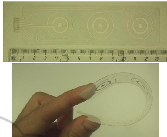
Figure 3: Implemented flexible array of three TCB concentric ring electrodes.
