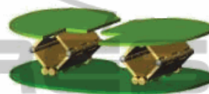
Figure 1: Example of use of the knee distractor instrumented with two scissor jack mechanisms (Marmignon et al., 2004).
