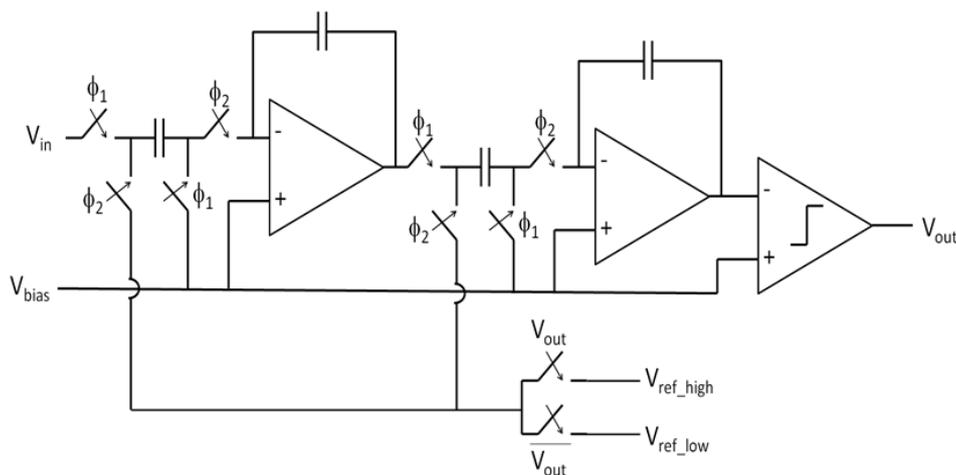
Figure 3: Top level modulator schematic.
