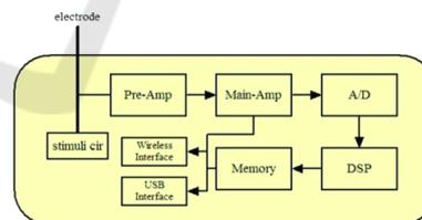
Figure 2: The top-level schematic of the biosensor system.
