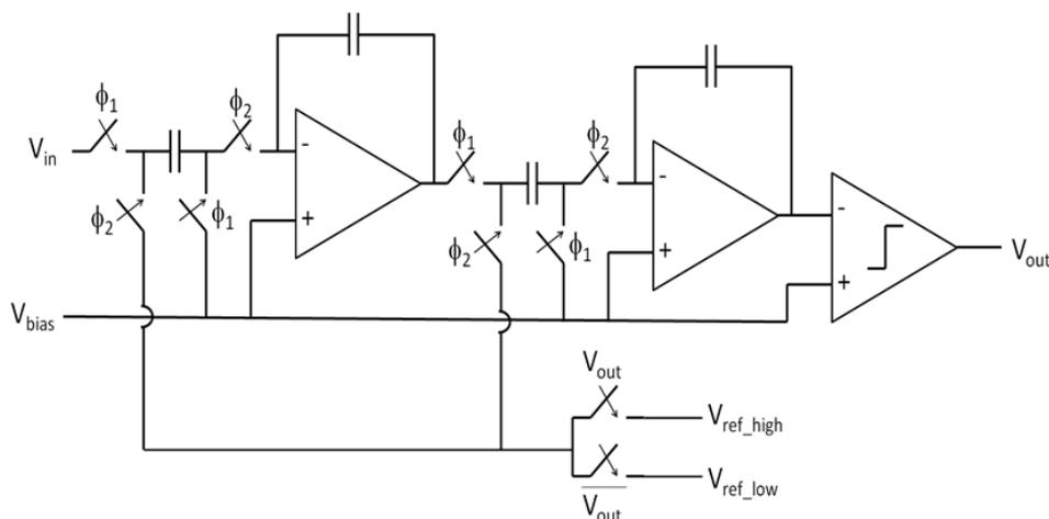
Figure 3: Top level modulator schematic.
