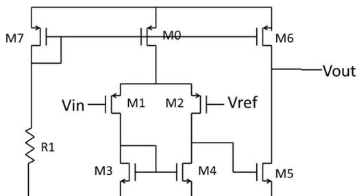
Figure 5: Comparator schematic.
