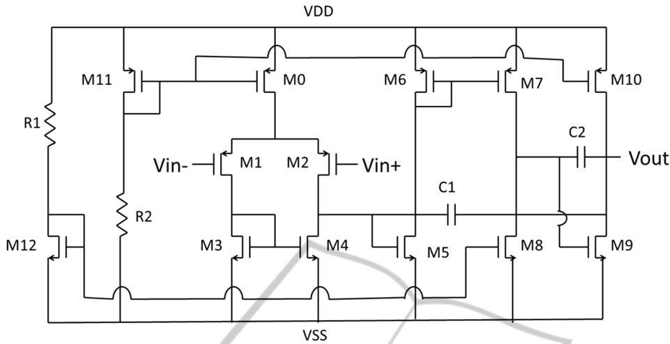
Figure 4: Op-amp schematic.
