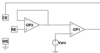
Figure 1: Potentiostat schematic.
