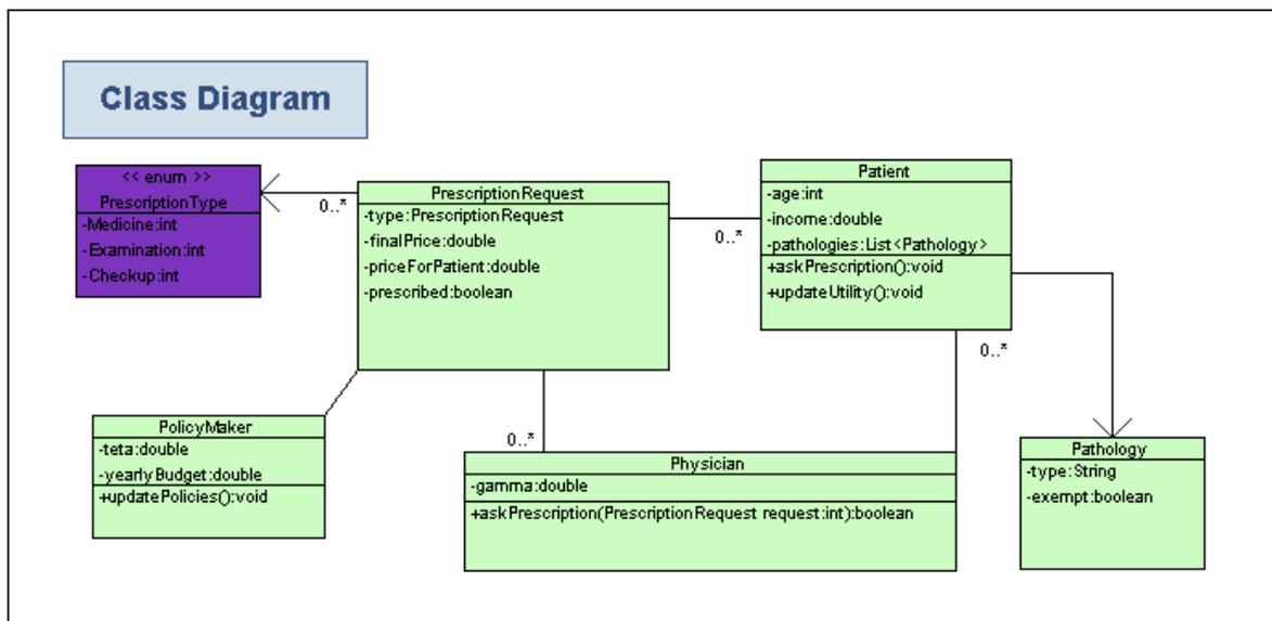
Figure 2: Class diagram of the model.
