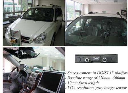
Figure 5: Our experimental vehicle and system.
