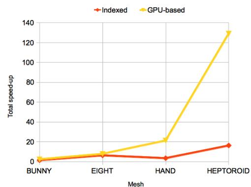
Figure 10: Speed-up factors for the time to convergence compared to the Sequential implementation.
