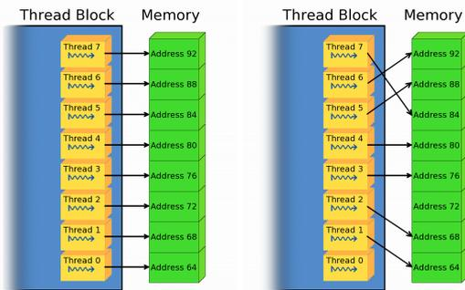
Figure 2: A coherent memory access from a block of threads, compared to an incoherent one.
