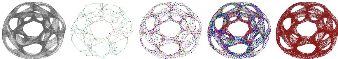
Figure 3: The SOAM (Piastra, 2009) reconstructs a surface from the point cloud on left. At the end, all units converge to the same stable state.
