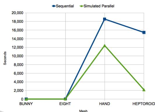
Figure 11: times to convergence of the Sequential and Simulated parallel implementations.
