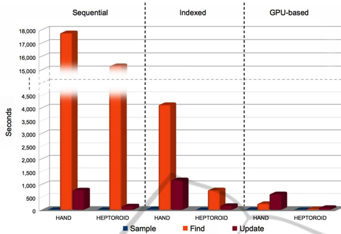
Figure 6: Single-phase time to convergence for the two more complex meshes in the test set.
