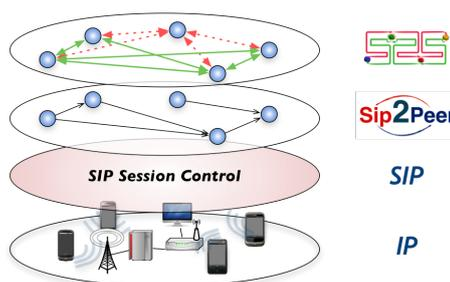
Figure 1: Communication stack.
