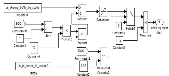
Figure 4: Charge torque required.
