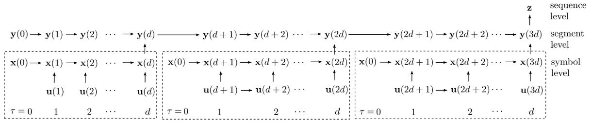
Figure 2: SMRNN dynamics for a sequence of three segments with fixed interval  $d$ . Processing on symbol level is described by Eq. 1 and illustrated in the dashed squares. The segment level above, is processes as described by Eq. 2. Finally, Eq. 3 describes how the network output  $z$  is obtained for the sequence.
