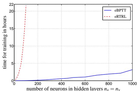
Figure 4: Computation time for training depending on the number of neurons in the hidden layers of the network. Training lasted 100 epochs of 50 sequences of length  $T = 60$ .
