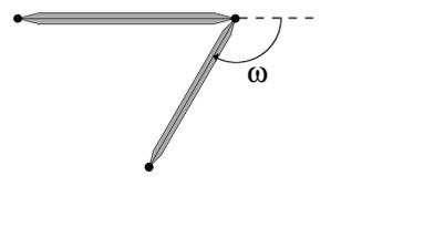
Figure 1:  $\rho = 2^{1/3}$  and  $\omega = 2\pi/3$ . We have a full-extension configuration, i.e.,  $e_1 = e_2 = 1$ , and the rotation controls  $r_1 = 0$  and  $r_2 = 1$ . In particular  $r_2 = 1$  implies that the angle between the first phalanx and the second phalanx is  $\pi - \omega = \pi/3$ .
