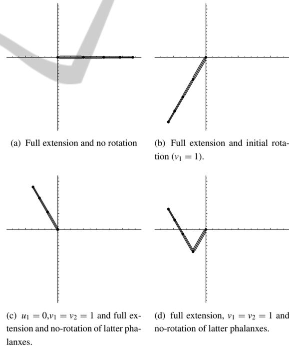
Figure 3: Extremal configurations for  $R_4(2^{1/3}, 2\pi/3)$ .
