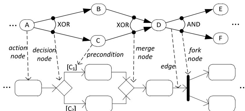
Figure 4: Example of TFM to Activity diagram transformation.
