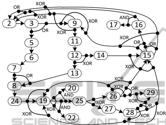
Figure 3: TFM representing enterprise data synchronization system functioning and logical relations between cause-and-effect relationships.
