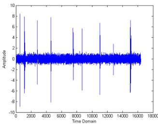
Figure 2: An example of spread spectrum signal with mixed Gaussian and impulse noise in the time doamin.
