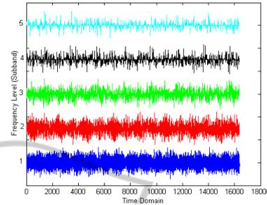
Figure 7: Mixed Gaussian and impulse noise suppression in the wavelet domain.
