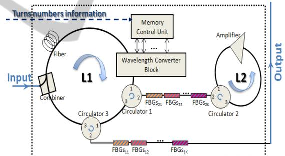
Figure 1: Multi-wavelength virtual memory architecture.
