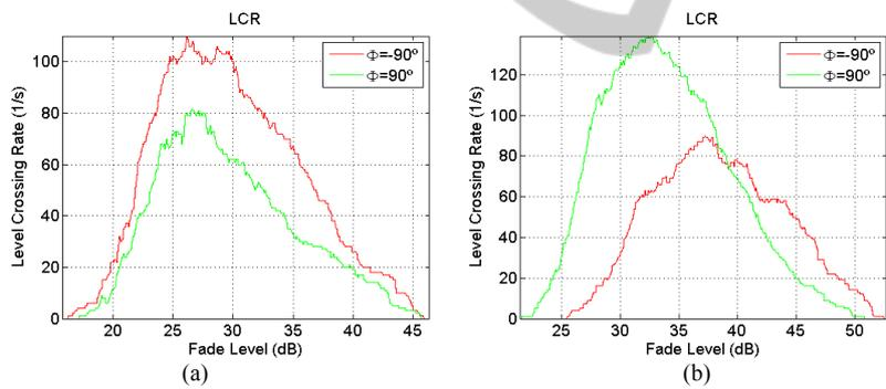
Figure 4: Measured LCR statistics at  $\phi=-90^\circ$  and  $\phi=90^\circ$ , for wind incidences from: a) B and b) F.
