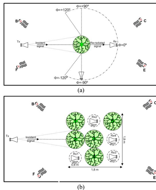
Figure 1: Measurement geometry of the: a) single tree and b) tree formation scenarios.
