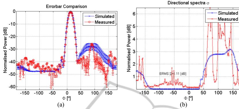
Figure 11: Comparison between measured and simulated data from position Rx1, with wind incidence C, considering: a) directional spectra errorbar and b) directional spectra standard deviation.
