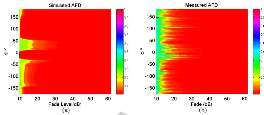
Figure 14: Comparison of data from position Rx2, with wind incidence E, between: a) simulated and b) measured data sets.
