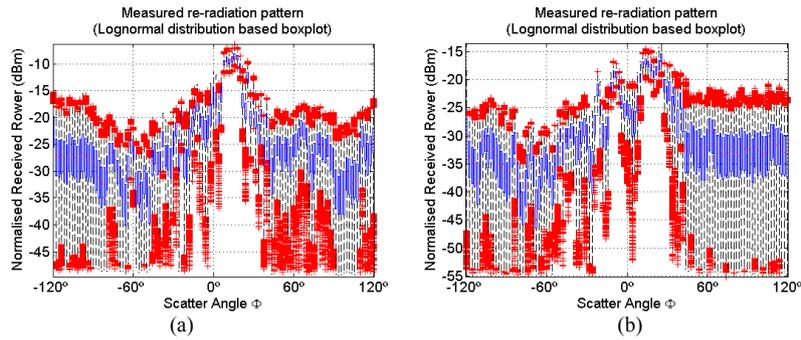
Figure 2: Measured re-radiation boxplot patterns for wind incidences from: a) B and b) F.
