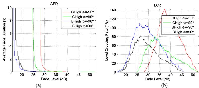
Figure 5: Measured statistics at  $\phi=-90^\circ$  and  $\phi=90^\circ$ , for wind incidences from B and C, concerning: a) AFD and b) LCR.
