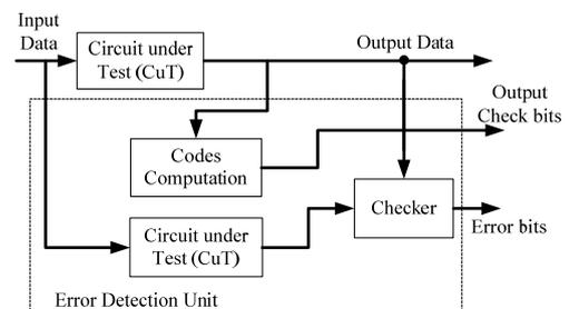
Figure 3: Block diagram of a TSC based on DWC.
