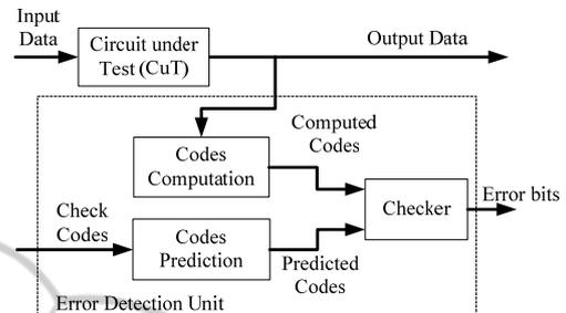
Figure 2: Block diagram of a TSC component based on information redundancy.
