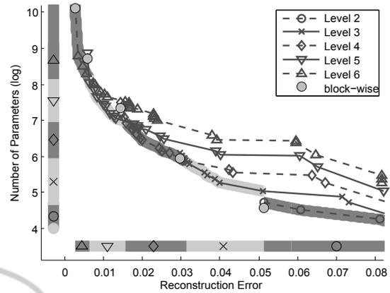
Figure 3: Number of parameters depending on the reconstruction error for different segmentation levels. The algorithm using the affine motion model was applied to the car sequence.
