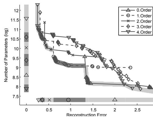
Figure 5: Number of parameters depending on the reconstruction error for different models. The algorithm segmented to the fifth level was applied to the hand sequence.
