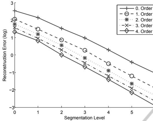
Figure 2: Mean value of the reconstruction error depending on the segmentation level for two optical flow datasets. Each curve shows a different motion model.
