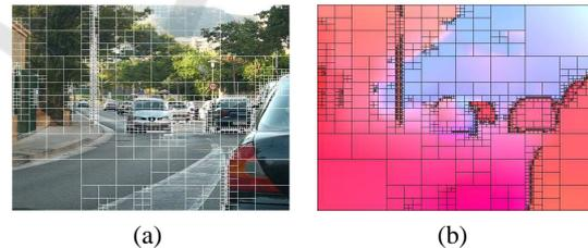
Figure 1: On the left is an example image and on the right the corresponding color coded flow field. The color value codes the moving direction and the intensity the amplitude of the motion. The lines show the quadtree segmentation.
