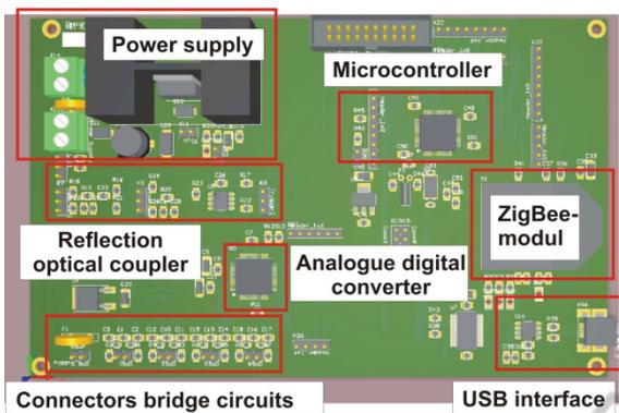
Figure 3: Interface electronics, PCB-layout.
