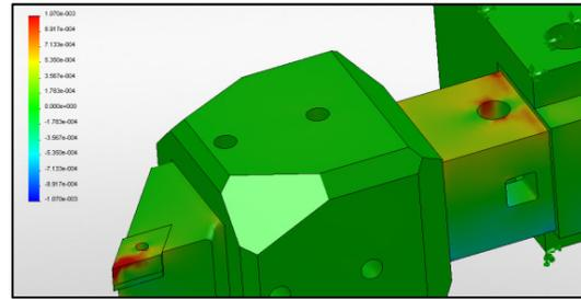
Figure 2: X-component of strain ( $F_c = 1200$  N).
