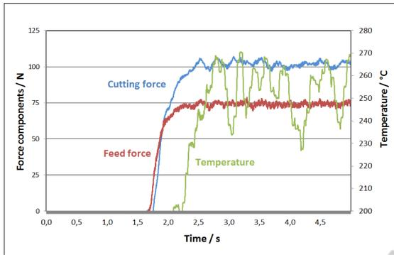
Figure 6: Cutting force, feed force and temperature, straight turning of titanium alloy with carbide inserts.
