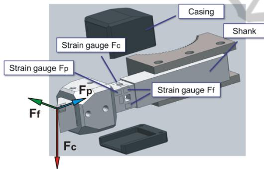
Figure 1: Dynamometer with strain gauges.
