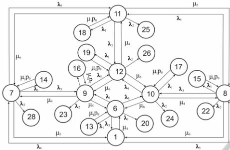
Figure 4: States graph of Markov chain for description of GCC failures while spacecraft remains reliable (state 1).
