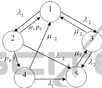
Figure 1: States graph of Markov chain for the simplified model of a technological control contour.
