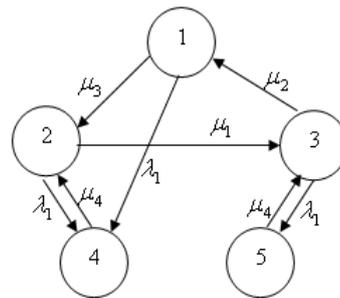
Figure 2: States graph of Markov chain for simplified model of command-programming control contour.
