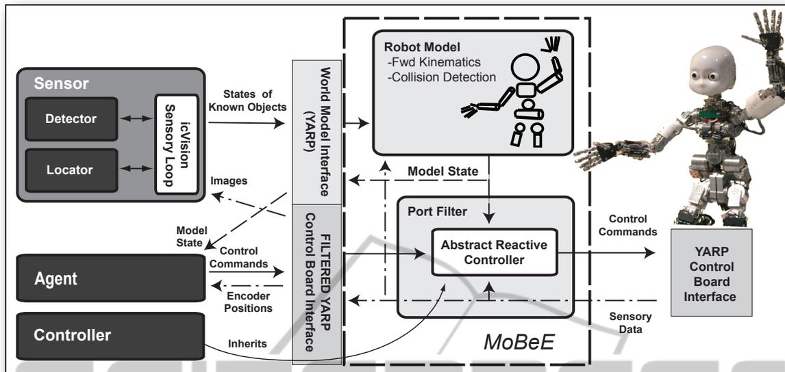
Figure 1: Simplified architecture of the MoBeE system - The Sensor, the Agent and the Controller (left), interact with the iCub humanoid robot through MoBeE. The iCub's behavior is decomposed and represented in terms of three weakly coupled behavioral modules, the Sensor, (composed of the Detector, the Locator) the Agent, and the Controller.
