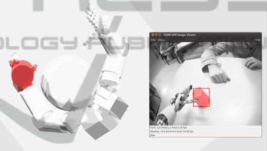
Figure 8: The resulting pose after reaching to the cup using an integrated Sensor, Agent, Controller system with the iCub robot. The inset (right) shows the iCub’s vision, overlaid with the (red) output of an Detector module. The cup, modeled as a cylinder, has been placed into the MoBeE model (left) by a Locator module. The roadmap used to plan the reach is pictured in figure 7.
