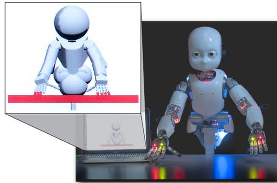
Figure 2: The kinematic model within MoBeE detects impending collision between the iCub's fingers and the table. Colliding geometries are rendered in red.
