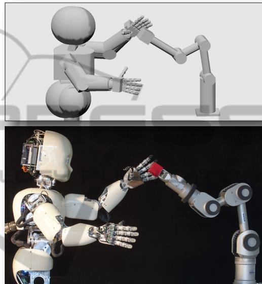
Figure 6: The iCub and Katana robots (bottom) cooperate in a shared workspace. Each robot is controlled via its own Agent/Controller pair and the shared MoBeE framework (top).
