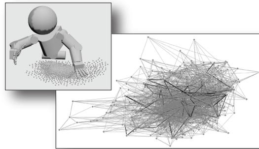
Figure 7: A large roadmap is constructed by searching the configuration space for a set of approximately 5,000 “interesting” poses. The scattered dots in the robot model (top-left) represent the position of the left hand as the robot assumes the pose associated with each vertex in the map (bottom-right).
