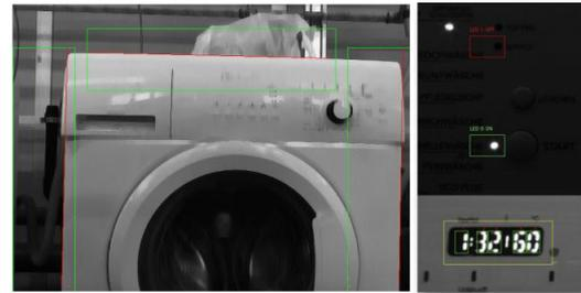
Figure 5: WM edge recognition (left) and panel inspection (right).
