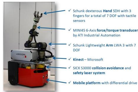
Figure 1: Overview of the developed mobile service robot.
