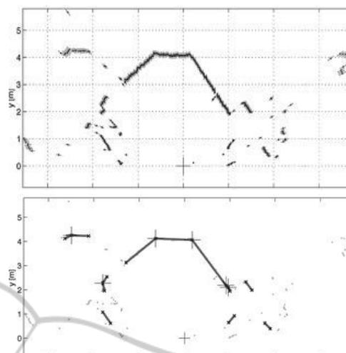
Figure 3: Data processing for lines extraction (upper: raw data, lower: processed data).
