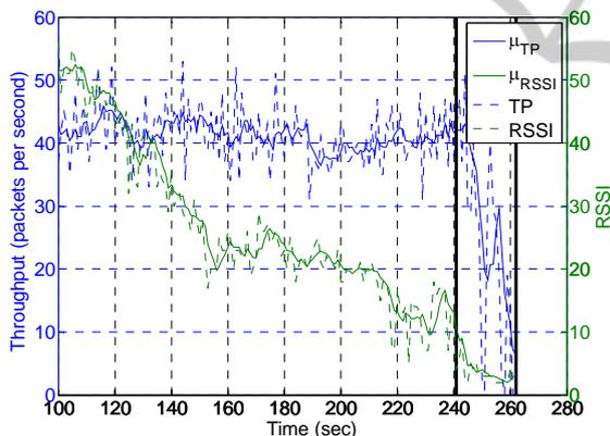
Figure 3: Example of video throughput (blue) and RSSI data (green) received at the OCU from a *PackBot* using the MDCR system. Solid line is the average ( $\mu$ ) of past five samples of underlying (dotted) data. Left and right black lines represent  $t_F$  and  $t_L$ , respectively.
