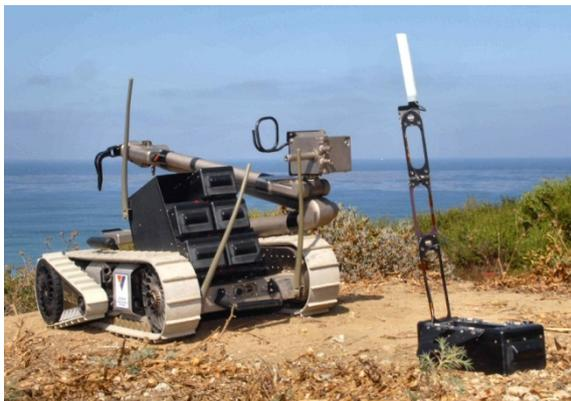
Figure 1: ADCR Deployer mounted on an iRobot *PackBot* with one deployed and five stowed Relay Bricks.
