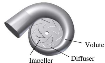
Figure 2: Centrifugal pump fluid domain.
