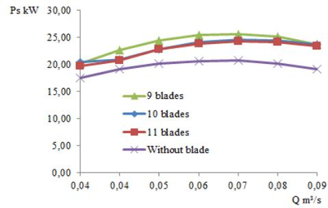
Figure 6: Brake horsepower versus volume flow rate.
