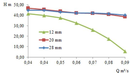
Figure 2: Pump head versus volume flow rate.
