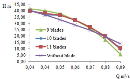
Figure 5: Pump head versus volume flow rate.
