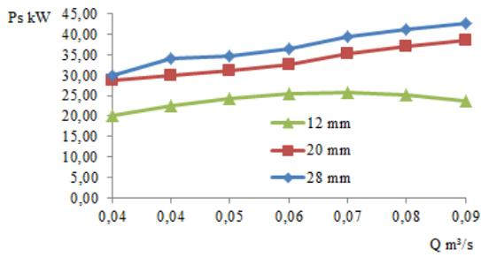
Figure 3: Brake horsepower versus volume flow rate.
