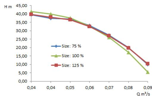
Figure 8: Pump head versus volume flow rate.
