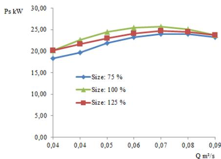
Figure 9: Brake horsepower versus volume flow rate.
