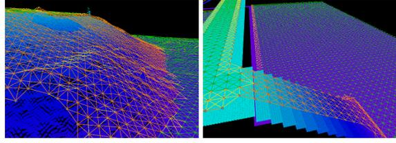
Figure 3: Examples of motion graphs for two different maps; left for a map of a training hill and right for an artificial urban map. The motion graphs encode whether the given robot model is able to traverse the terrain. Areas with risk values and slopes below a convenient level are green, areas with higher risk levels and convenient slopes are yellow, and areas with higher risk values and higher slopes are orange.
