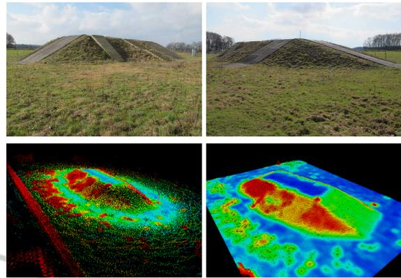
Figure 12: Second real-world scenario. The top row shows two images of the testing hill. In the bottom row the point cloud and the filled, smoothed map are depicted. The size of the map is  $43.95 \times 32.95 m$ . The colors indicate the risk of traversal, ranging from blue for flat regions over green and yellow to red, high risk areas.
