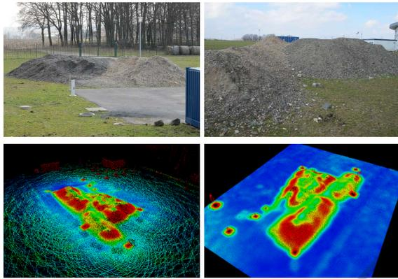
Figure 10: First real-world scenario. The top row shows two images of the hill of rubble. The bottom row depicts the point cloud and the filled, smoothed map. The size of the map is  $36.4 \times 30.45 m$ . The colors indicate the risk of traversal, ranging from blue for flat regions over green and yellow to red, high risk areas.
