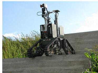
Figure 1: The Telemax robot model, a tracked platform with four actuators, enabling the system to overcome more complex obstacles than many other robot systems.
