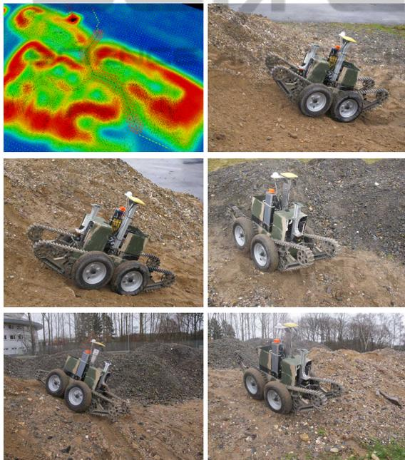
Figure 11: Results of the first real-world experiments. The first image depicts the plan given to the robot. The other pictures show the robot during the execution. If the robot safety permits, configurations are sometimes applied in advanced or while in motion to avoid stop-and-go movement.
