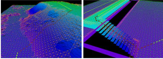
Figure 4: Path segments of the initial paths for two planning queries on different maps. Segments through flat regions which do not require further planning are shown in light green, segments through rough regions will be refined in the second planning phase and are shown in dark red.
