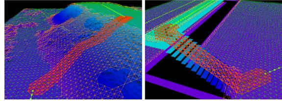
Figure 5: Two examples of tubes (light red) around the initial paths in rough areas. The tubes are used to restrict the search space of the detailed motion planning step.
