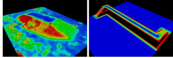
Figure 2: Risk distributions of two different maps; left of a real map build by a laser range finder and right for an artificial urban map. The risk of a region is based on the height differences in this area. The roughness quantification is used to control the planning process. The colors are indicating the degree of risk, ranging from blue for flat regions over green and yellow to red, high risk areas.
