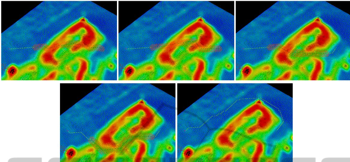
Figure 7: Influence of the safety weight of the initial path search. It determines the primary direction of the final path.
