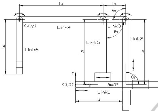
Figure 1: Schematic diagram of links for the finger-rehabilitation robot instrument.
